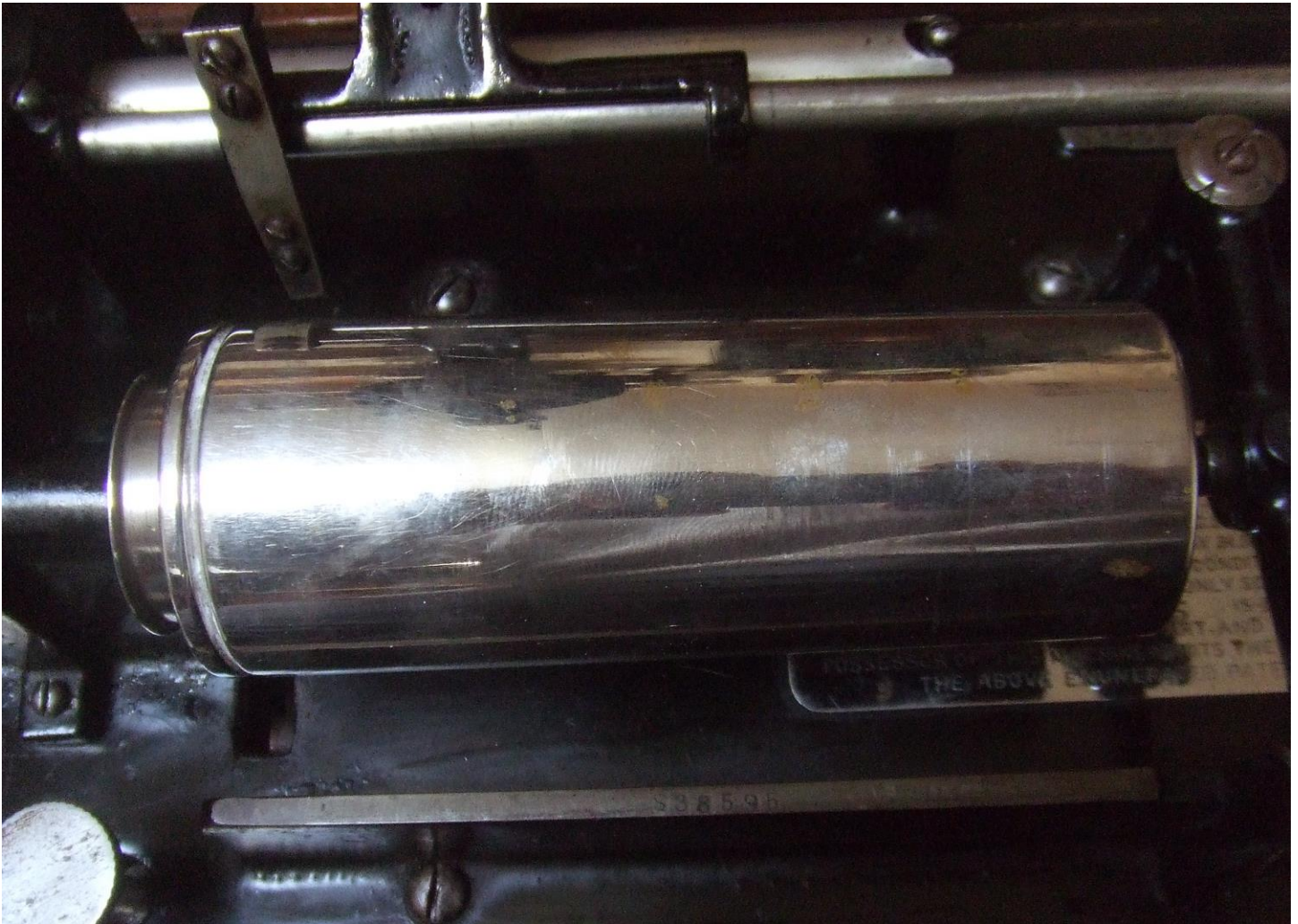
Late grooved mandrel – Photo courtesy of Alistair Sandilands
